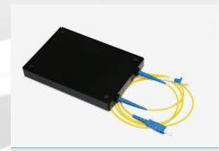
OTDR LAUNCH BOX An Optical Time Domain Reflectometer (OTDR) launch cable connects the OTDR to the fiber link under test. Its function is to overcome the "Dead Zone" which is caused by the near end reflection at the OTDR connector interface. Using a launch cable enables an accurate near end measurement of the input connector of the fiber link under test.
