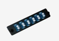
ADAPTER PANELS LITRA MFG's wide range of Adapter Panels are designed to fit the popular LGX footprint. SC adapters are available in 6-pack simplex and 12-pack duplex panels. LC adapter panels are available in 12-pack duplex and 24-pack quad versions. Adapter panels are also available for ST and FC connectors in 6- and 12-pack configurations. Adapter colors of green (APC), blue (SM) and beige (MM) are standard.
